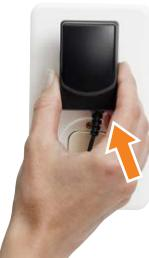
Plug the mains adapter into the mains socket.
